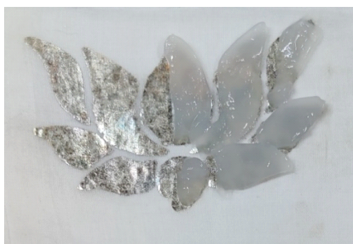
Figure 2: Opaque flexible gel of 0.75% high acyl gellan gum
