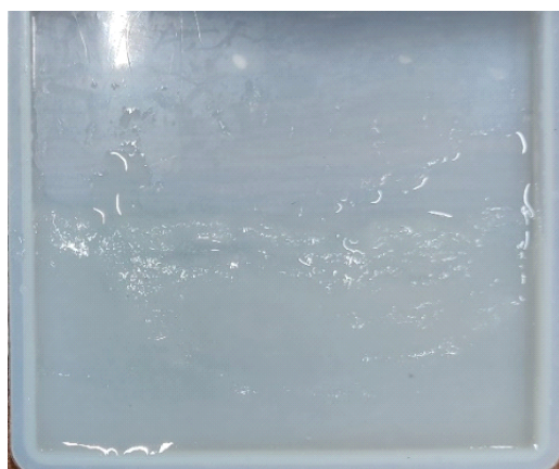
Figure 4: Gel not forming with triammonium citrate
